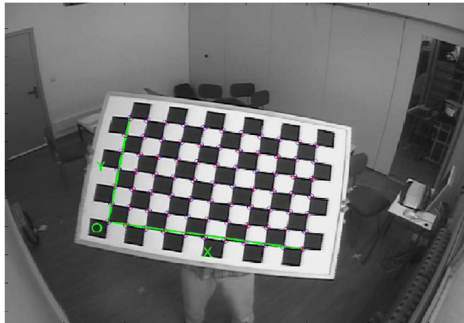
Figure 2.9: Calibration process of the cameras of the smart-room of our lab using a chessboard as the pattern of reference.
