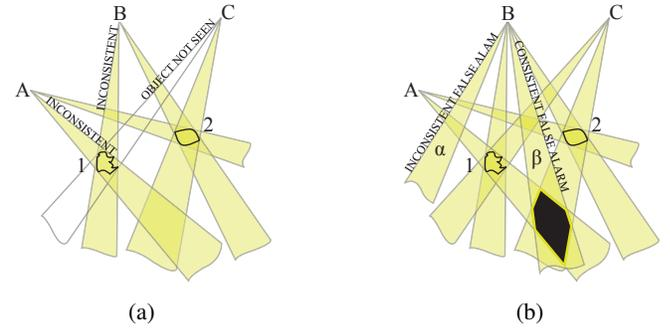
**Fig. 2.** In (a), object 2 is correctly detected in all the cameras, but object 1 is missed in camera C. The union of the cones  $camB \rightarrow obj1$  and  $camA \rightarrow obj1$  forms the IH. In (b) there have been two false region detections in camera B ( $\alpha, \beta$ ). The first one ( $\alpha$ ) forms an inconsistent cone, while the second one ( $\beta$ ) forms a consistent one for intersecting with other C-1 visual cones.
