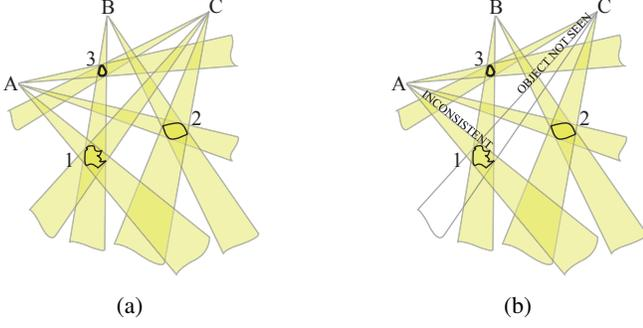
**Fig. 3.** In (a), objects 1, 2 and 3 are correctly detected in cameras A, B and C. In (b), object 1 is not reconstructed. The IH is smaller than its counterpart in Fig. 2 due to the occlusion of object 1.
